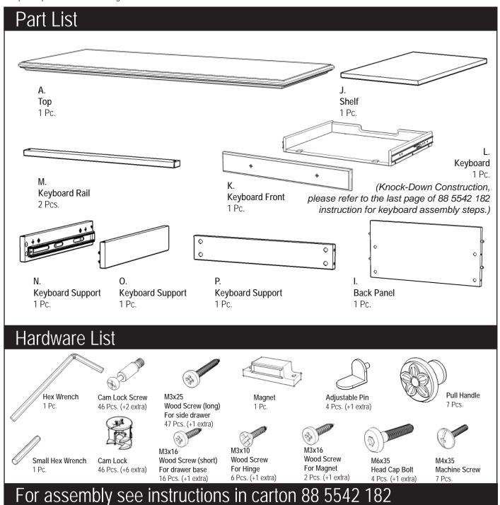
Tools required for assembly : Phillips screwdriver
